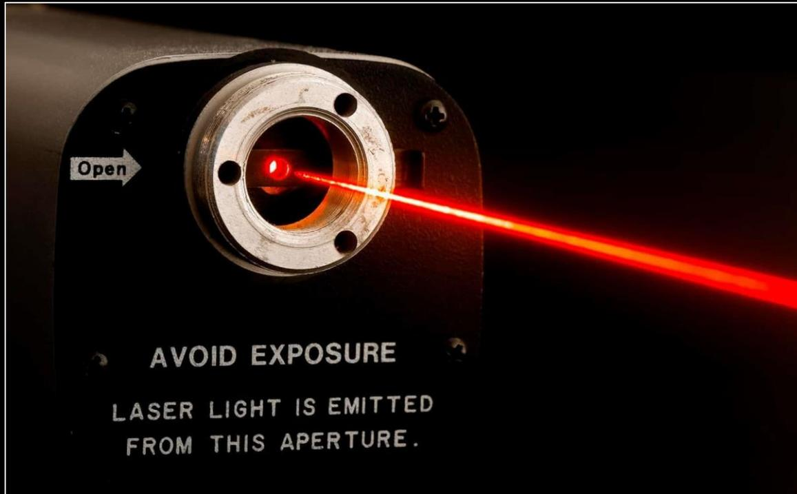
Le laser (light amplification by stimulated emission of radiation)
